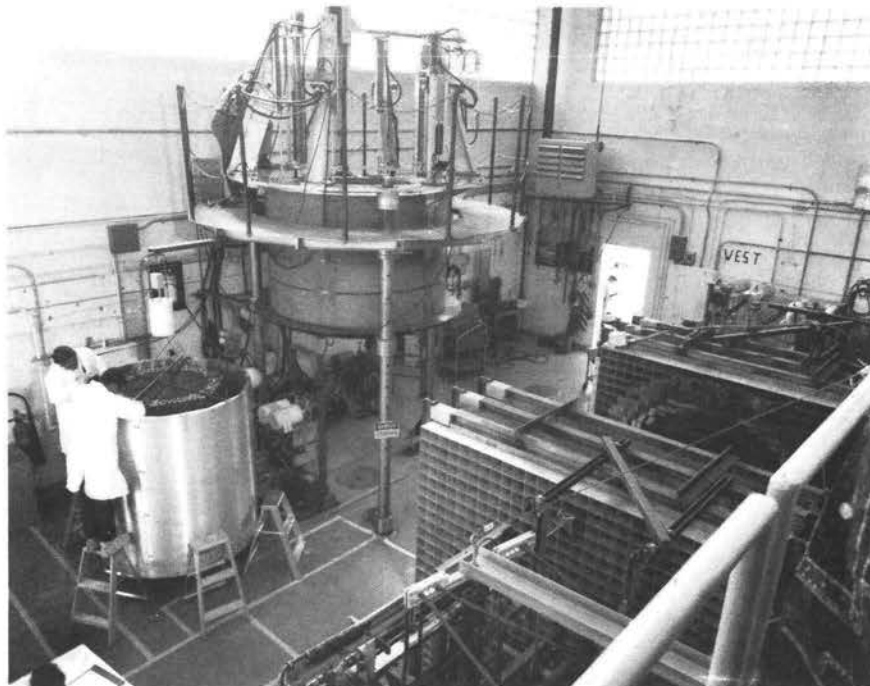
Fig. 20. The core, with 4000 fuel elements, being assembled in the zero-power mockup of the Phoebus-2 reactor. A much cruder simulation of the same reactor is in the Honeycomb machine at the right.
