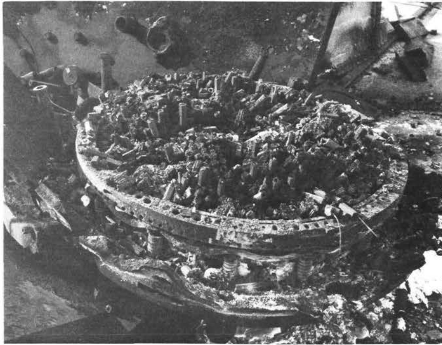
Fig. 18. Remnant of Kiwi-TNT on test stand after the planned destructive excursion.
