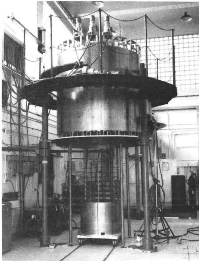
Fig. 23. A beryllium-reflected cavity assembly set up in Kiva 1 as a preliminary to the Plasma Core Assembly.
